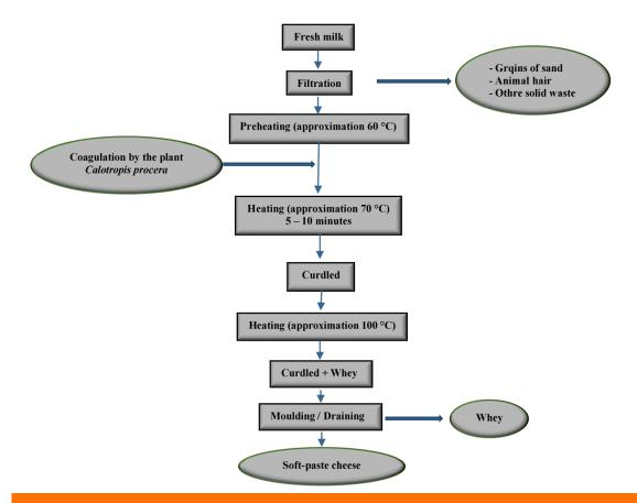
Figure 1. Typical diagram of *Peulh* cheese making (Dossou *et al.*, 2006)
