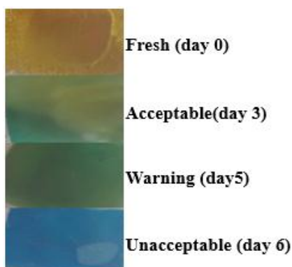
Figure 3. Range of the color change in the indicator at different days: Yellow, fresh; yellowish green, acceptable; blue, unacceptable.
